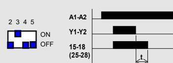
The function can be inverted with switch 2 = ON.
