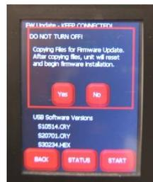
Once the firmware files are transferred to the VMX-synergy™ unit, the update process will commence. The update process is a three-step process indicated on the touchscreen. Once the update is complete, VMX-synergy™ will reboot and display the status
