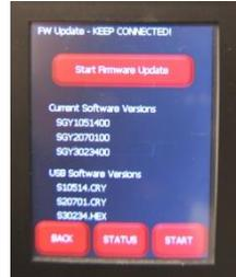
Confirm the firmware update by pressing YES. Ensure the VMX-synergy™ unit remains powered during the update process.
